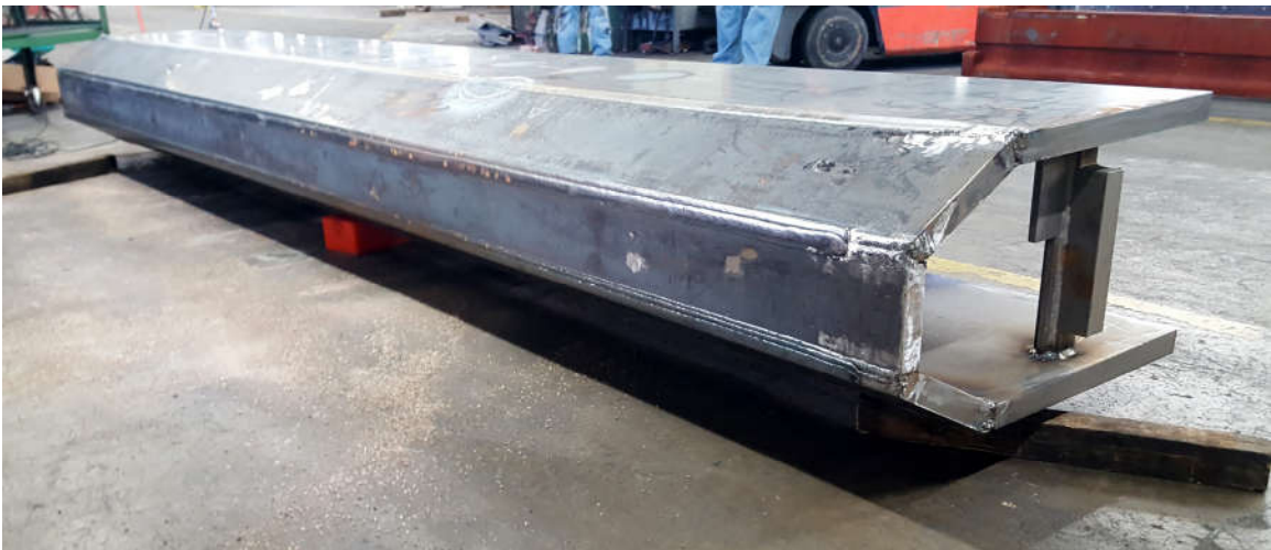
Figure 9 shows back of head structure, with single cushion at the center. Again, this arrangement of 3 cushions positioned far from the corners of the workpiece allows the flexure to occur that is critical to achieving effective stress relief.
