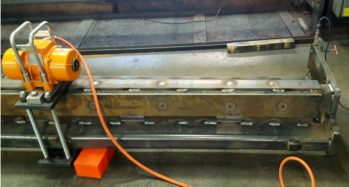
Figure 2: VSR Tooling consisted of two plates, each with a 4 bolt pattern for the threaded rod, plus 2 mounting holes for the vibrator. Accelerometer is on right.
