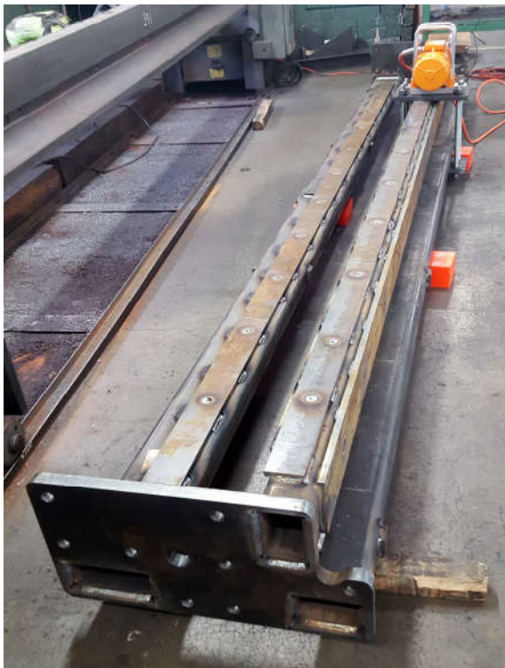
Figure 1: Frame setup for VSR Treatment. Three isolation cushions are positioned around the center of the frame, separated by ~ 5 feet, with the vibrator near the far cushion. This cushion arrangement minimizes damping, and thus maximizes workpiece resonances. An accelerometer is mounted on the far left corner, and oriented to be most sensitive to vertical amplitudes. Note that the vibrator's AOR (Axis of Rotation) is aligned with the workpiece length, which allows both vertical and horizontal amplitudes to be generated.
