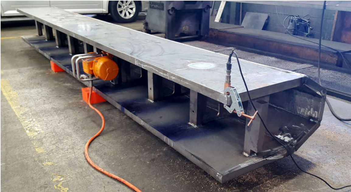
Figure 8: Workpiece # 2 / head structure was setup in a manner similar to # 1. An adapter plate was used to secure the vibrator using the bolt pattern in the cross-brace. Two treatments were performed, again a high-frequency range, with modest unbalance setting, and a low-frequency range treatment, with higher unbalance setting. This approach assures that all the available modes of vibration, and hence, flexure patterns, are treated.
