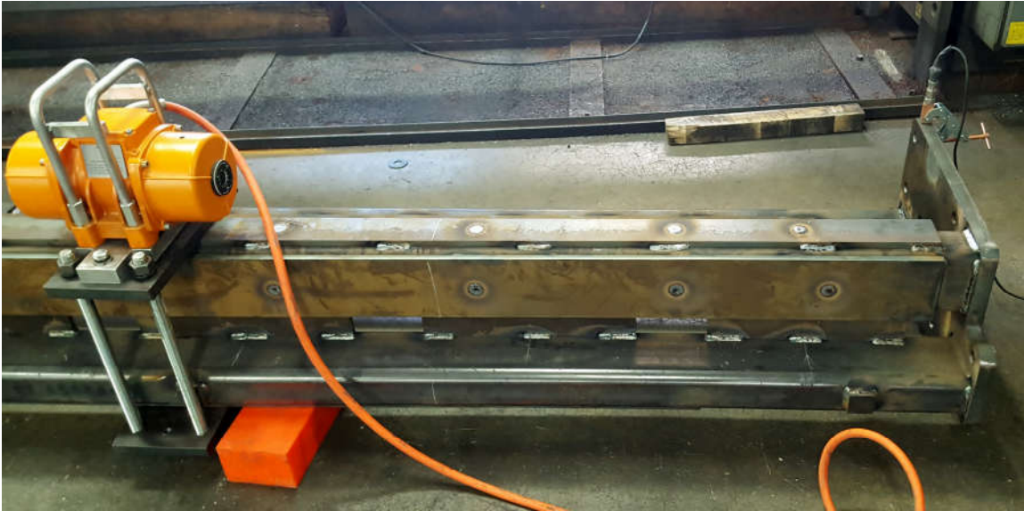
Figure 2: VSR Tooling consisted of two plates, each with a 4 bolt pattern for the threaded rod, plus 2 mounting holes for the vibrator. Accelerometer is on right.
