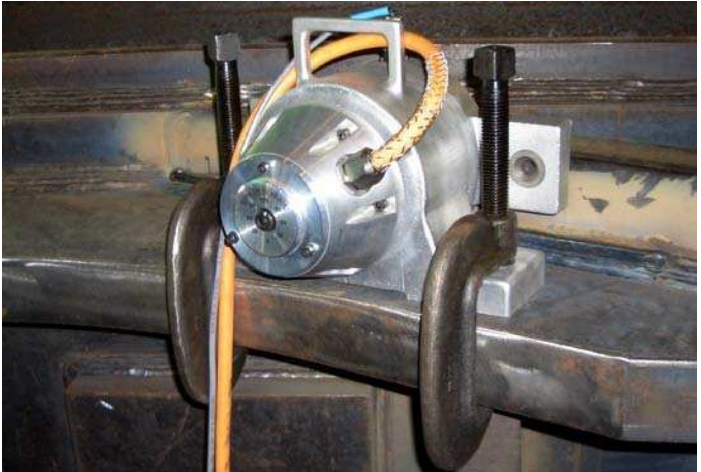
Figure 4: Close-up of System's BL8 Vibrator. This Vibrator has adjustable speed (10 – 8,000 RPM) and adjustable unbalance (0.2 – 4.0 in-lbs.), the unbalance scale is visible on the back of the vibrator. It also features two sets of mounting feet, so that it can be oriented most effectively. Hardened steel inserts (Rc 50) in the mounting feet allow strong, effective clamping, without crushing the aluminum-magnesium alloy housing. Vibrator is driven by a 3 HP ( \approx 2.3 kW) brushless DC motor.
