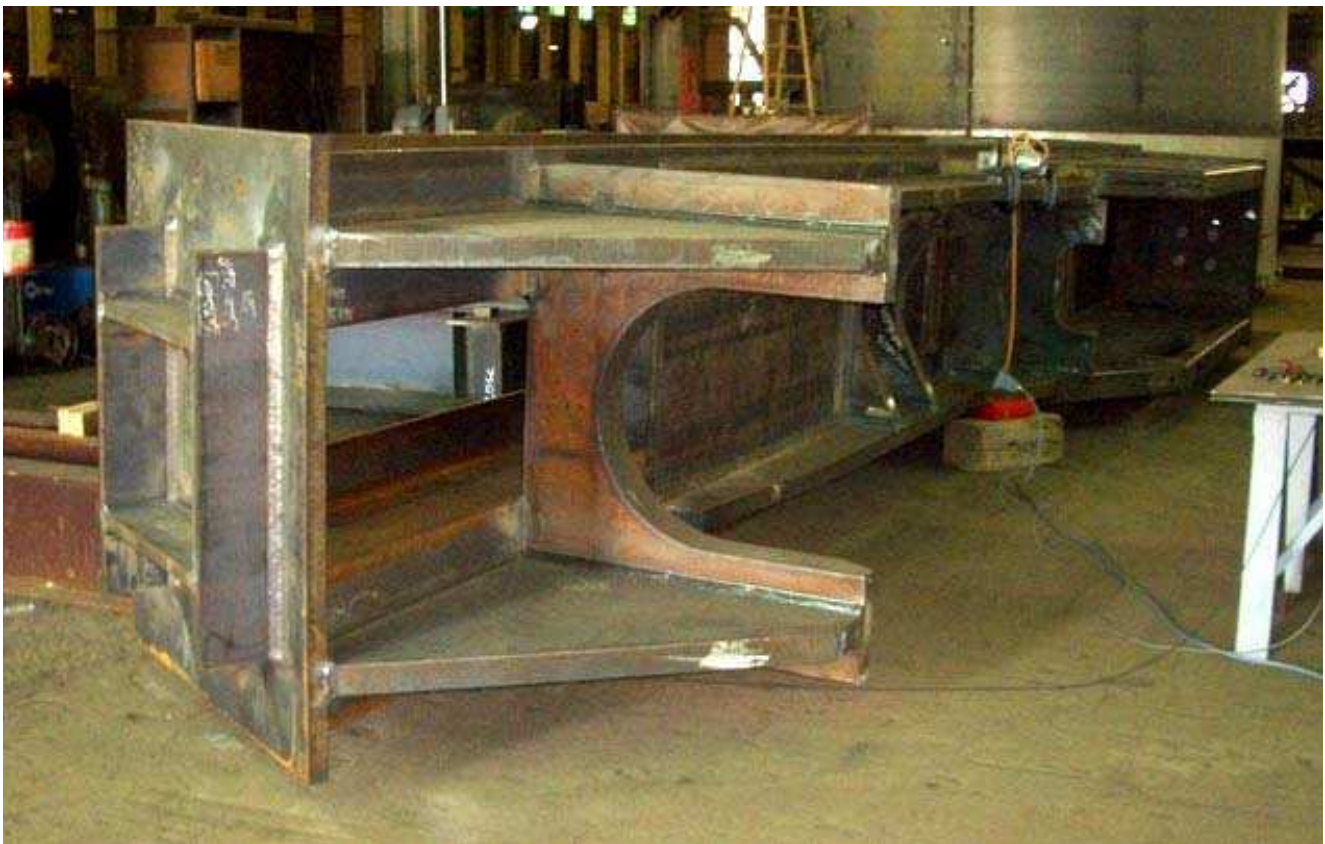
Figure 1: View from near one end of the 30-ton Ingot Stripper Frame. The Frame was isolated on 3 Isolation Load Cushions (1 is visible), midway down the length of the Frame). Each Load Cushion was placed on a 10" X 10" wood block to achieve leveling and floor clearance (Frame is \approx 4" above the floor in the foreground.) The BL-8 VSR Vibrator, clamped to the Frame, can be seen directly above the Cushion.
