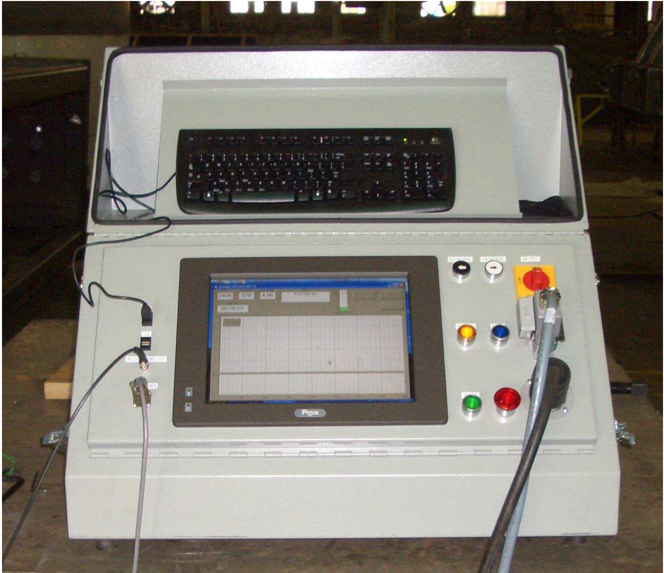
Figure 6: MX-8000 VSR Console. Touch-screen computer displays VSR Scan Data, digital data (RPM, power, and acceleration). Scan data is saved in Adobe/pdf format. Low voltage connections are on left (2 USB Ports, Accelerometer, and Vibrator resolver / tachometer), and higher voltage connections on right (power in, motor).
