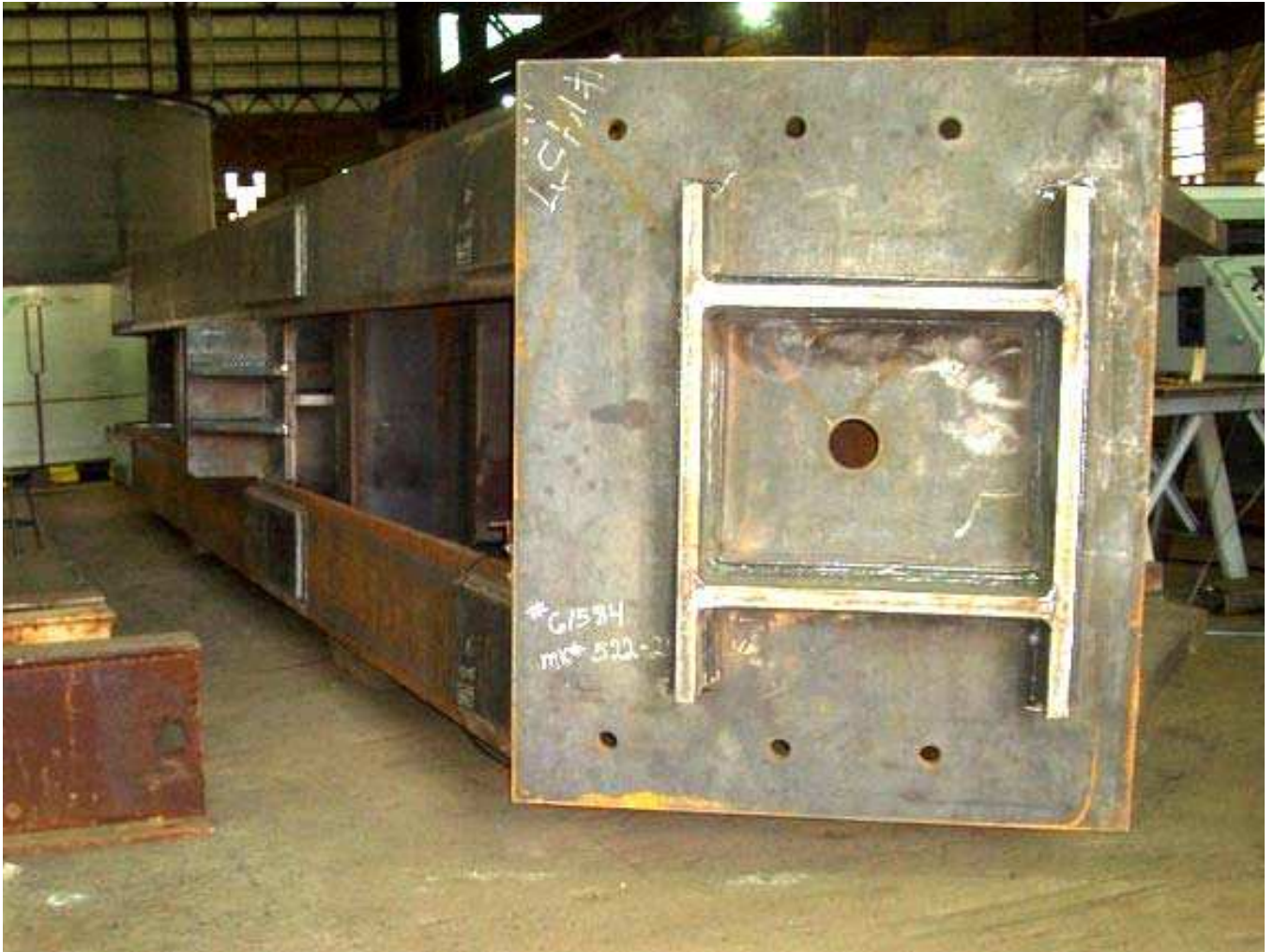
Figure 2: View showing opposite side that shown in Figure 1. Note the two wood blocks spaced at the 1/3rd points along the length. These leveling blocks hold the other 2 Cushions. This 3 point Cushion arrangement minimizes the damping of the Frame during Treatment, allowing effective resonating to take place, which produces the flexure required for the VSR Process. The Accelerometer Clamp and cable is visible on the near left corner (circled).
