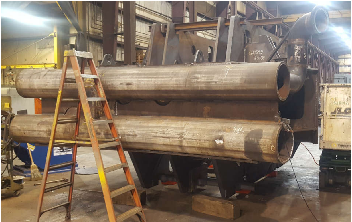
Figure 3: View from other side of shows accelerometer mounted on lower tube, oriented to be most sensitive to vertical amplitudes.
