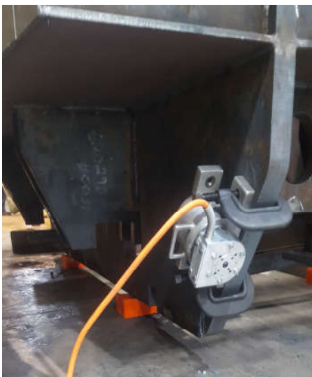
Figure 1: Workpiece was placed on four urethane isolation cushions, positioned to minimize the damping of the structure, and thus promote resonance, a key requirement of the VSR Process. Vibrator is seen in the lower left corner, where it was during the first VSR Treatment. The accelerometer (vibration sensor) was placed on the far corner from this view, and oriented to be most sensitive to vertical amplitude.
