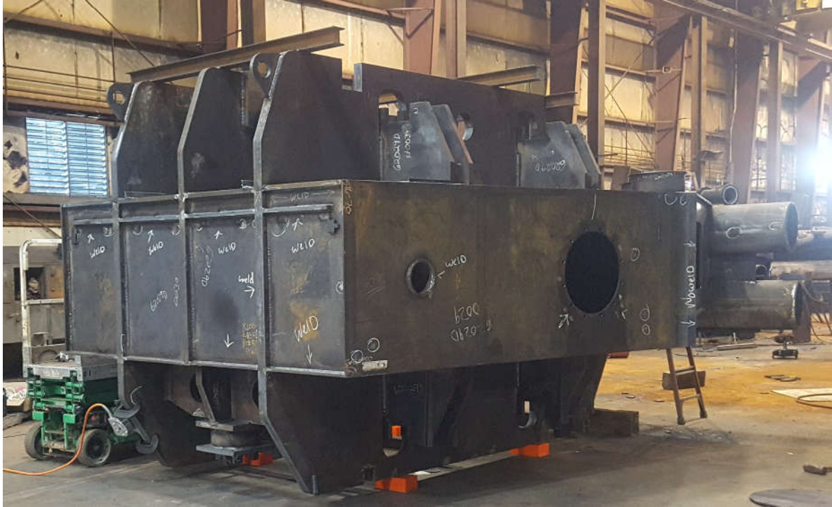
Figure 1: Workpiece was placed on four urethane isolation cushions, positioned to minimize the damping of the structure, and thus promote resonance, a key requirement of the VSR Process. Vibrator is seen in the lower left corner, where it was during the first VSR Treatment. The accelerometer (vibration sensor) was placed on the far corner from this view, and oriented to be most sensitive to vertical amplitude.
