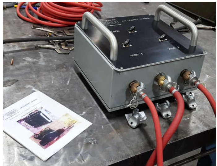
Square tubing fabrication distortion was reduced by a factor of SEVEN TIMES using the 3D Pneu Drive VDW System. First welding jig for robotic assembly station suffered 7/16" / 11 mm distortion. Thereafter, VDW technology controlled distortion to less than 1/16" / 1.5 mm
