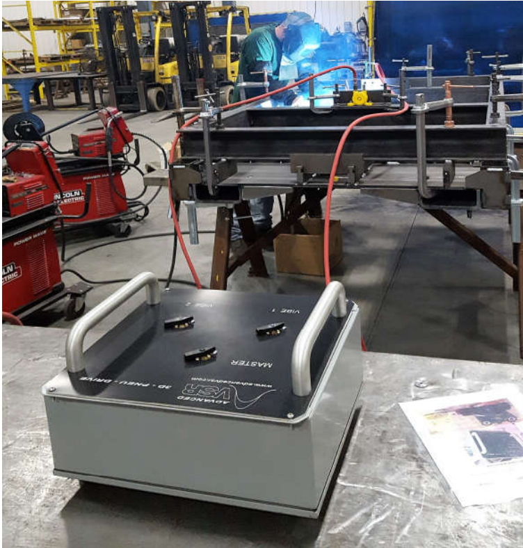
VDW System controlling distortion of precision skids for use in robot cells for automotive industry.
