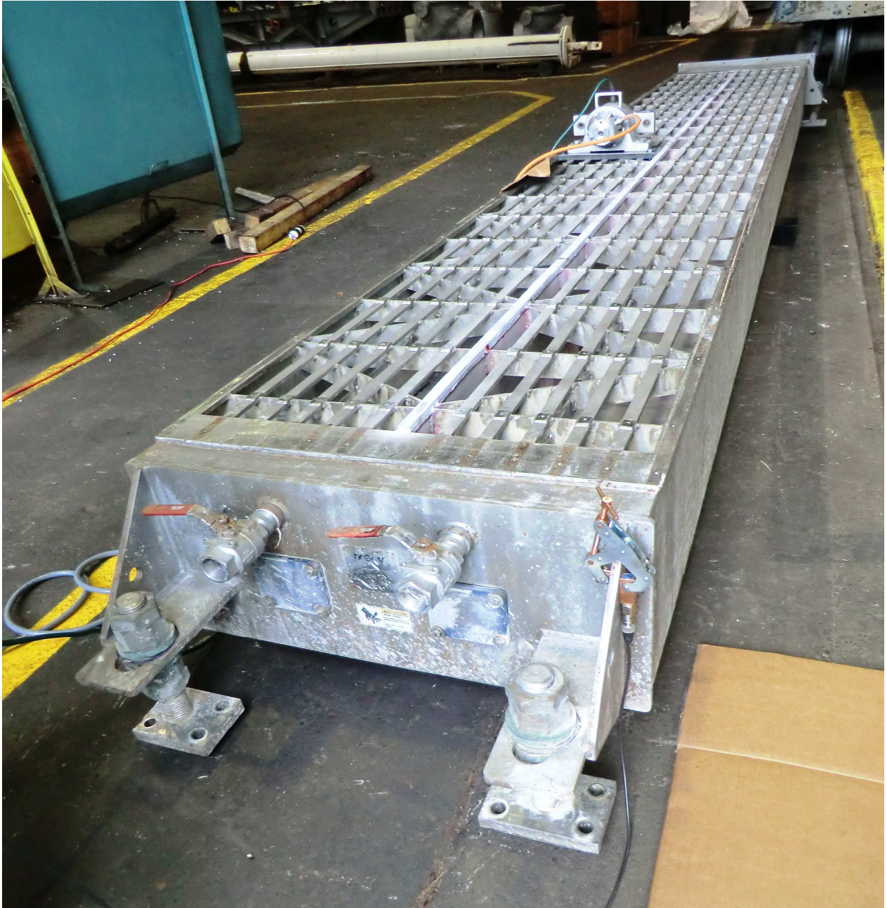
Figure 4: View from the end of the workpiece shows accelerometer in right-foreground, and single isolation cushion on the right, at the midpoint of the workpiece length.
