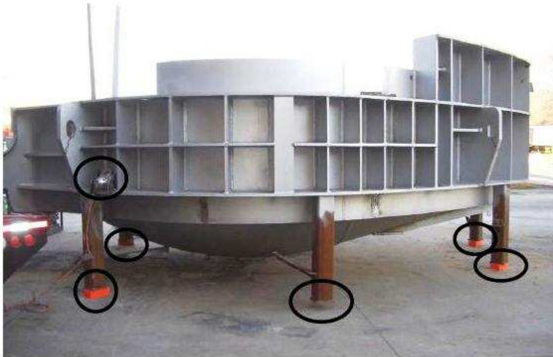
Figure 1: VSR Setup. Four Isolation Load Cushions (circled) supported the workpiece. The Vibrator was mounted on the left (circled), adjacent to one of the support legs. The Accelerometer (vibration sensor) was mounted on the opposite side of the workpiece, mounted to a protruding member, and oriented so as to be most sensitive to vertical deflection.
