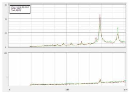
Pre-Treatment Scan shown on left provides the all the information needed by the operator to perform the VSR Process.
