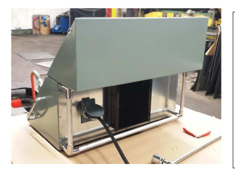
Closer view of powder-coated console enclosure, rear view shows drive heat sink and power inlet, both protected by an aluminum and stainless steel cage. Heat sink dissipates more than 85% of drive generated heat, keeping all electronics (drive, PC, power supply, etc.) subjected to minimal heat stress.
