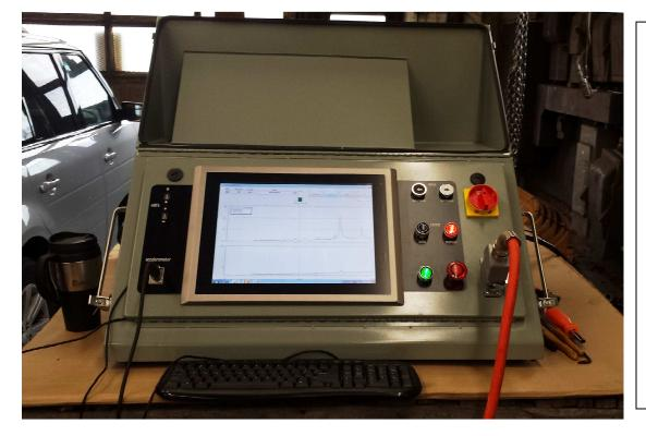
A-VSR MX-8a Console displays the clear vibration data needed to perform the VSR Process effectively.
