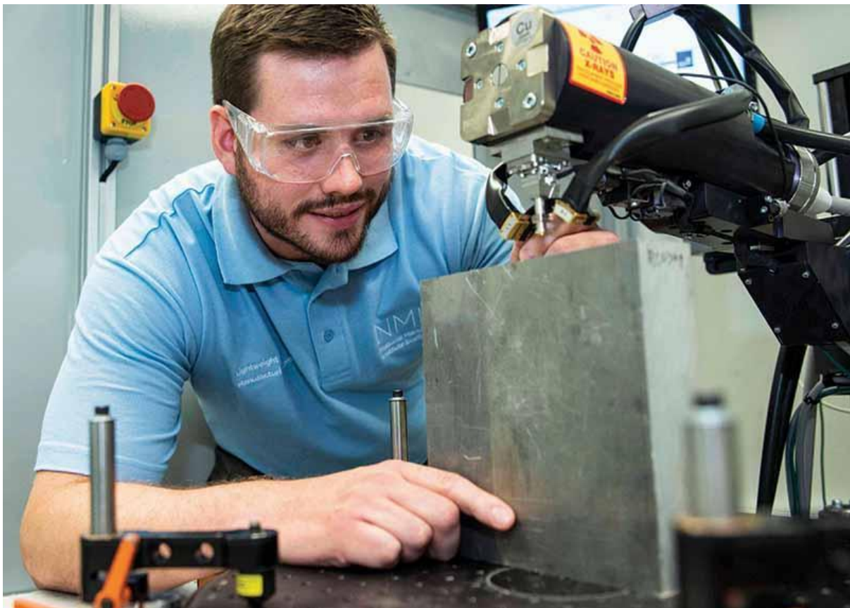
Dr David Easton with X-ray diffraction machine used to measure residual stress in a part © National Manufacturing Institute, Scotland
